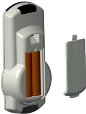
To insert the batteries, pull out the plastic flap of the dedicated compartment, making a little pressure over the cleats and sliding the flap down. Then insert 2x1.5V AAA batteries paying attention to the direction, indicated inside the body, close the door by inserting it from the bottom and pull it up until you can hear the joint.
