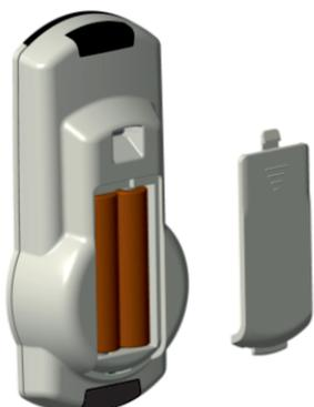
To insert the batteries, pull out the plastic flap of the dedicated compartment, making a little pressure over the cleats and sliding the flap down. Then insert 2x1.5V AAA batteries paying attention to the direction, indicated inside the body, close the door by inserting it from the bottom and pull it up until you can hear the joint.
